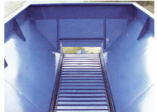
Heavy-Duty Hopper Construction With Heavy-Duty Chains.
