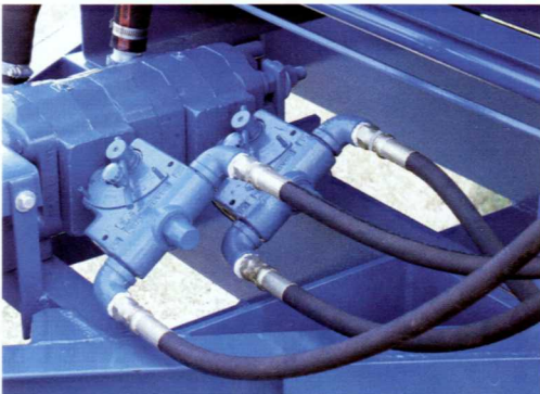
Optional Self-Contained Or Plug to Tractor Hydraulics
